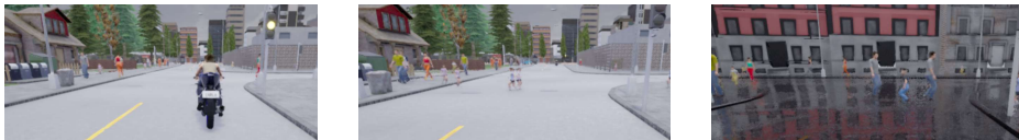
Figure 3: New types of vehicles and pedestrians present on the updated version of the benchmark. Left: motorbikes were not included on the previous benchmark. Middle: kids are now also part of pedestrians. Right: now pedestrians are able to better agglomerate when crossing roads.
