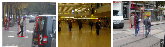
Figure 7: Some detections of the HOG method in the INRIA dataset. The blue BBs are the groundtruth and the red ones are the detections.
