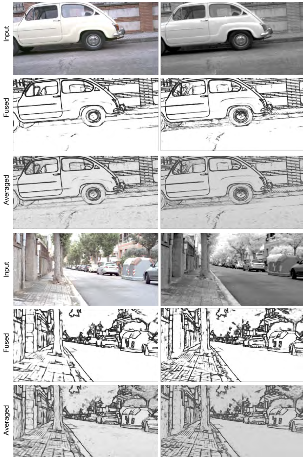
Fig. 5. Illustration of edges extracted in two pairs of images. (Input row) RGB and NIR images. (Fused row) Edge maps corresponding to fused predictions ( \hat{y}_i^{(fso)} ) by HED ( left-side ) and MSI-HED ( right-side ). (Averaged row) Edge maps corresponding to averaged predictions ( \hat{y}_i^{(av)} ) by HED ( left-side ) and MSI-HED ( right-side ).
