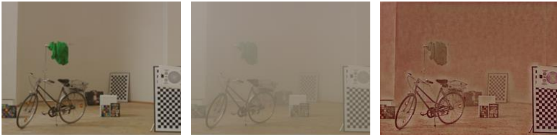
Figure 5. (left) Real clear image; (middle) Real haze image; (right) Result from the Two Branch network trained from scratch with Lüthen et al. dataset.
