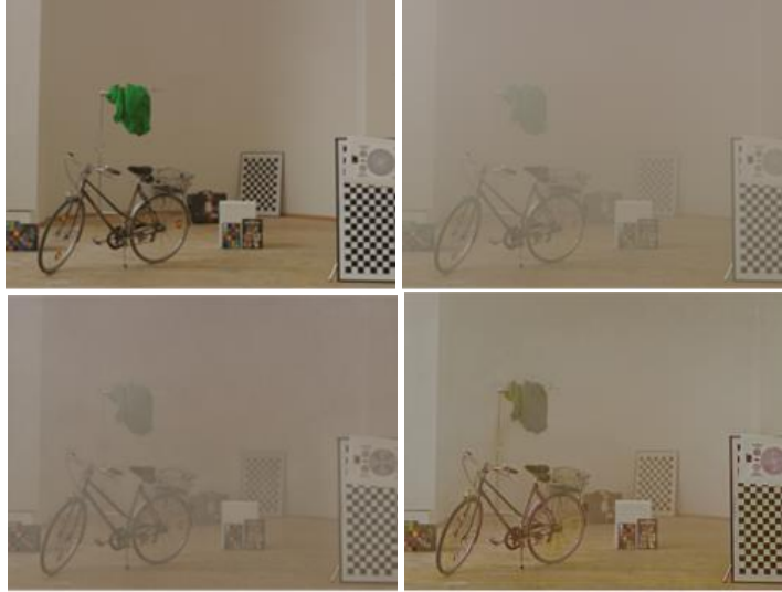
Figure 6. ( top-left ) Real clear image; ( top-right ) Real haze image; ( bottom-left ) Result from the Two Branch trained with our synthetic dataset. ( bottom-right ) Result from the Two Branch trained with our synthetic dataset and fine-tuned with Lüthen et al. dataset.
