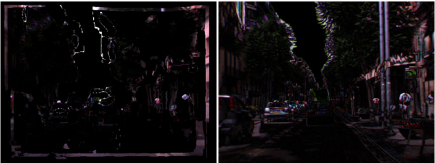
Fig. 4 ( left ) D_{(u,v)} map of moving regions, from frames ( n ) and ( n+1 ) presented in Fig. 1 ( top ). ( right ) Image difference between these consecutive frames: (|\mathbf{I}^{(n)} - \mathbf{I}^{(n+1)}|) to illustrate their relative displacement.
