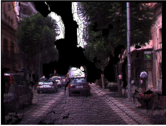
Fig. 2. Synthesized view representing frame (840) in the coordinate system of frame (841), by using the computed 3D rigid displacement: [\mathbf{R}_q | \mathbf{t}_q] .
