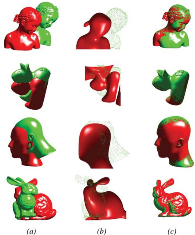
Fig. 8. Public data sets (from [27] and [28]) registered with the proposed approach and state of the art techniques. (a) Initial set up of the given source and target sets represented by means of triangular meshes to highlight details. (b) IPs representing target sets and source points. (c) Results of the proposed registration approach represented through triangular meshes to make visual evaluation easier.
