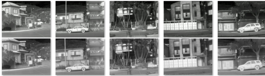
Fig. 2. Examples of thermal images. ( top ) MR images from Axis Q2901-E. ( bottom ) HR images from FC-6320 FLIR [Rivadeneira et al., 2020a].
