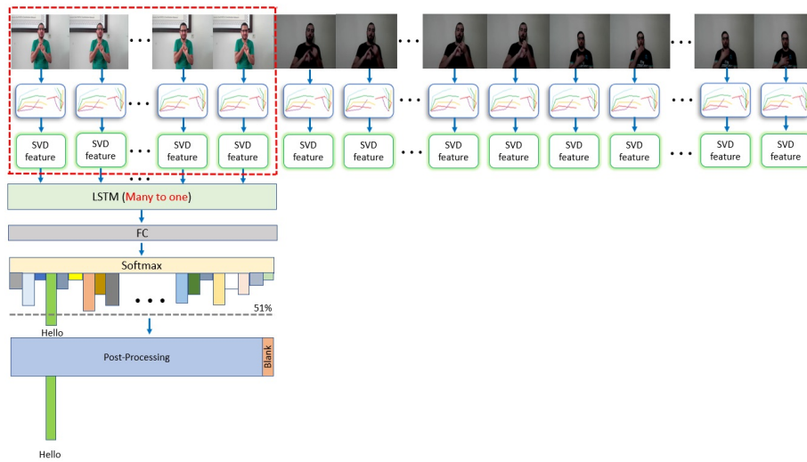
Figure 4: The first recognition of the "Hello" sign, which post-processing algorithm accepts it.
