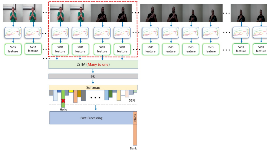
Figure 6: The post-processing algorithm assigns a “Blank” label if all outputs of the Softmax layer are less than 0.51.
