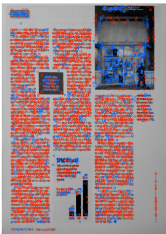
Fig. 1. Illustration of CORE filtering with SIFT (keypoints+features) for p = 0.01 and \sigma = 32.125 on SmartDOC dataset sample (magazine002). Blue and red points are respectively kept and discarded keypoints.
