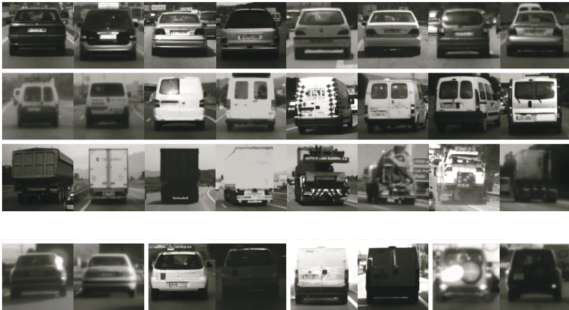
Fig. 1. Top) Heterogeneity of the objects to be detected, just from their rear-view. Bottom) Pairs of the same vehicle, acquired under different illumination conditions.
