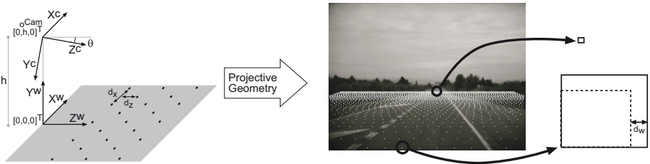
Fig. 3. Frame Scanning Process. For each inspected road point, rectangular regions of different widths and aspect ratios are evaluated.
