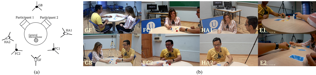
Figure 1. Recording environment. We used six tripod-mounted cameras, namely GB : General Rear camera, GF : General Frontal camera, HA : individual High Angle cameras and FC : individual Frontal Cameras, and two ego cameras E (one per participant, placed around their neck). a) Position of cameras, general microphone and participants. b) Example of the time-synchronized 8 views.
