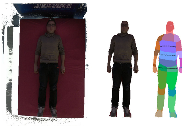
Fig. 12 Test under low-light conditions. First image shows the complete scene. Second image depicts the segmented body. The last image represents the segmented body parts with the computed body circumferences
