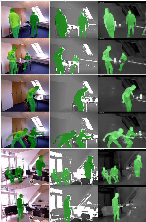
Fig. 7 Examples of the annotated imagery for two views in each of the three scenes. The RGB modality is manually annotated and the corresponding mask is registered to the depth and thermal modalities. The causes of registration misalignment of the masks are motion blur and noisy depth information, which induce parallax in the thermal modality
