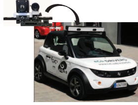
Fig. 4. Acquisition system (cross-spectral stereo rig on the top left) and electric vehicle used as mobile platform.
