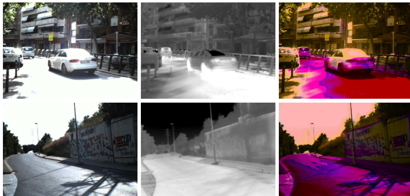
Fig. 3. Illustration of monochrome threshold based image fusion. ( left ) VS image. ( middle ) LWIR image. ( right ) Fused image.
