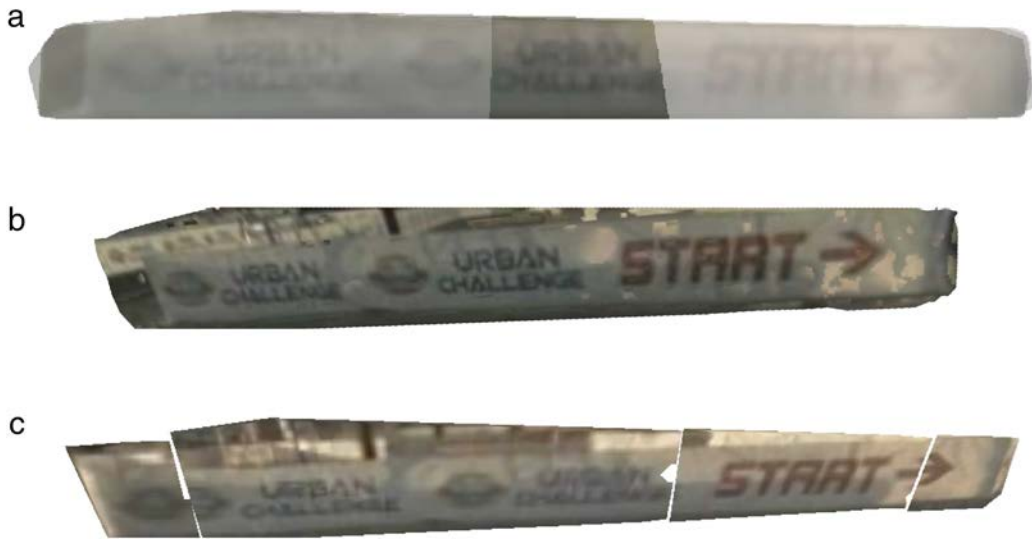
Fig. 3. Textures obtained using different fusion strategies: (a) option (1), average textures from local meshes; (b) option (2), insert vertices from all local meshes; (c) option (3), insert triangles of better quality, removing overlapping triangles.
