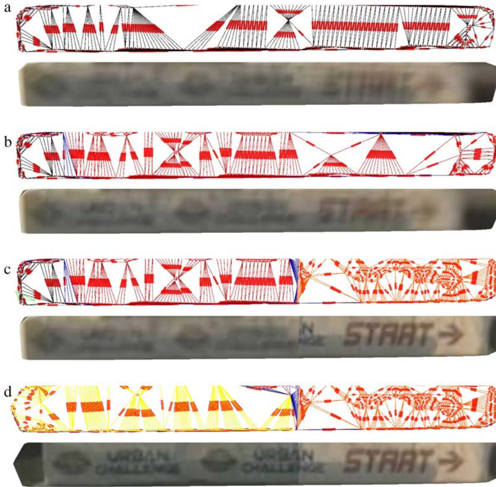
Fig. 10. The evolution of the global primitive mesh ( top ) as well as the texture ( bottom ): (a) time t = t_1 ; (b) time t = t_2 ; (c) time t = t_3 , insertion of front center camera; (d) time t = t_3 , insertion of front left camera. (For interpretation of the references to color in this figure legend, the reader is referred to the web version of this article.)
