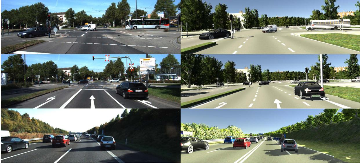
Figure 5: Images sampled from KITTI-Track (left) and Virtual KITTI (right). Note how Virtual KITTI is a synthesized but realistic clone of KITTI-Track.
