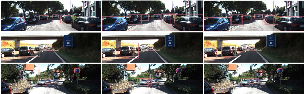
Figure 11: Vehicle detections when operating in the FPPI=1 regime. Left: DPM based on the SYNTIA data considered in this chapter (SRC). Middle: Using the TAR0.1 version of KITTI-Det Train. Right: Adapting SRC by using TAR0.1 when applying SA-SSVM.
