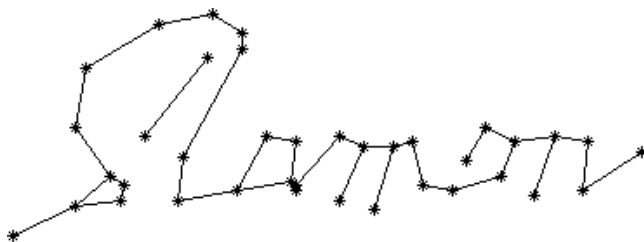
Fig. 5. Graph representation from the skeleton of a word. The critical points detected by the vectorization method are considered as the nodes and the lines joining them are considered as the edges.
