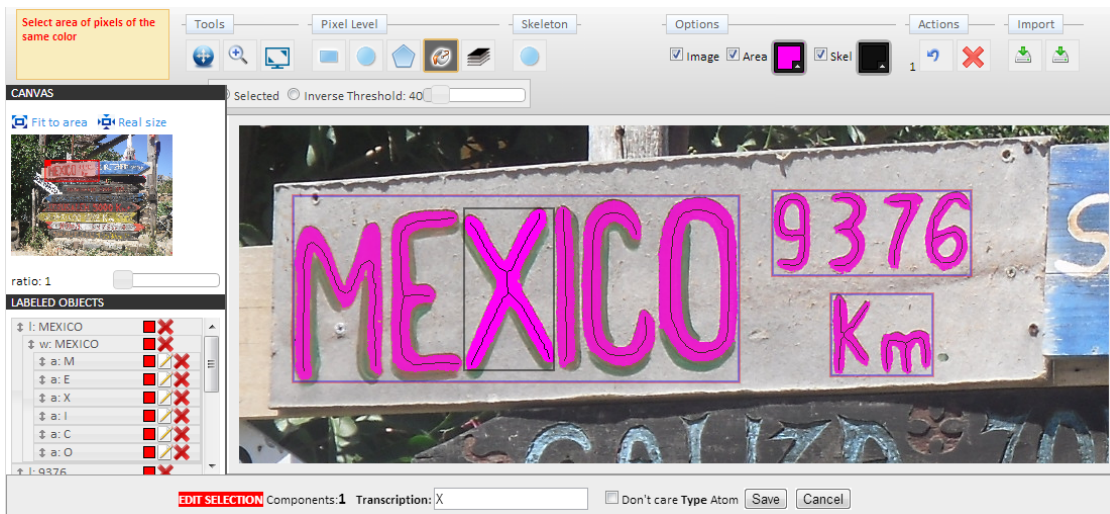
Fig. 1. A screenshot of the ground truthing tool, the hierarchy of textual content and the defined text parts (areas and skeletons) are visible over the image.
