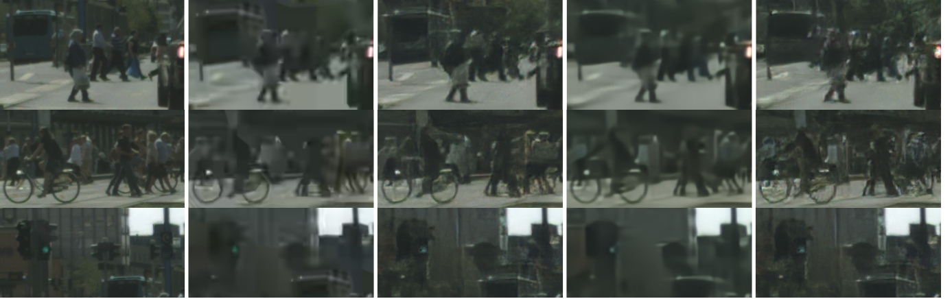
Fig. 2. Effects of compression and restoration (from left to right): captured image, compressed (BPG), restored (BPG), compressed (MSH), restored (MSH).
