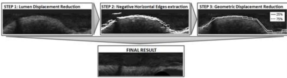
Figure 3.2: Scheme of the strategy for approaching the geometric center of mass
