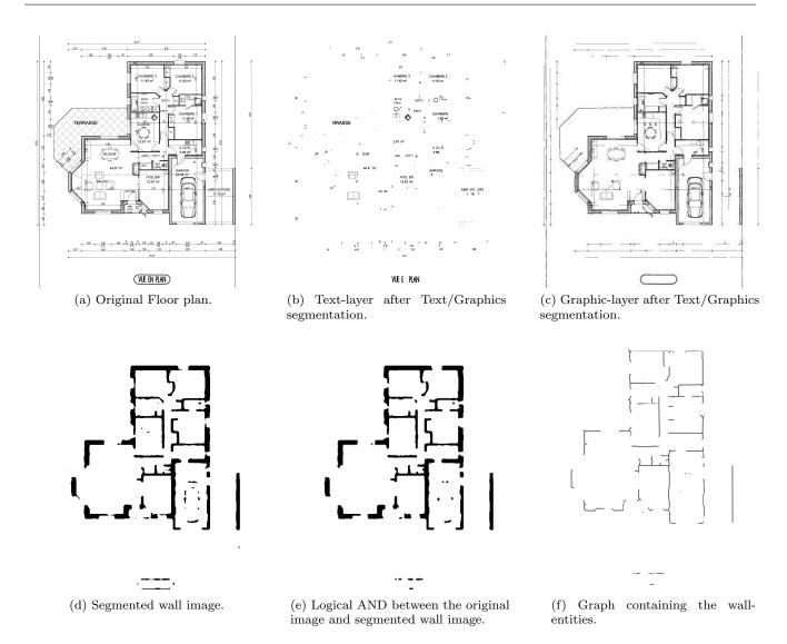
Fig. 3: Complete flow of wall recognition process.
