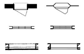
Fig. 6: Left: three different windows from real floor plans with dissimilar notations. Right: the respective vectorization. Black vectors belong to walls and gray to windows.
