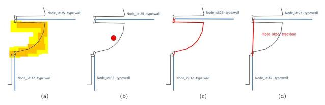
Fig. 7: Process for finding a door entity. In (a) shows the detection of the door by the statistical approach presented in Sect. 3 over the real image. The centroid of the area where the door is found is shown as a red point in (b). The node expansion by A\* for finding the path between the two walls in the graph is shown in red in (c). Finally, both walls are connected in (d) by means of a door node.
