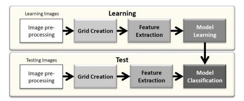
Fig. 2: Pixel-based segmentation pipeline.
