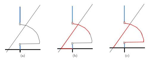
Fig. 8: A problematic situation is shown in (a) for finding door lines between the blue wall candidates. In this case a ceiling line traverses the door symbol. The nodes expanded (red) by a pure implementation of A\* algorithm in (b) shows that the final retrieved path does not traverses the complete door lines. Contrarily, in (c), additional cost for traversing wall nodes is added, and the final retrieved path is correct.
