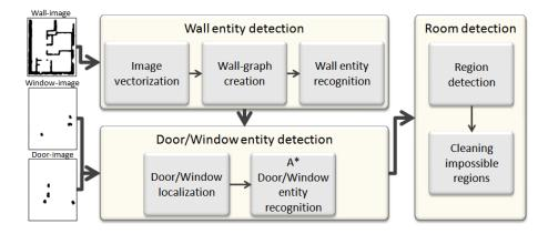
Fig. 4: Structural recognition pipeline
