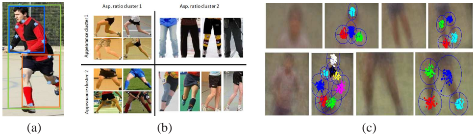
Figure 3: (a) Body joint annotations (blue stars) and different mid-level parts (bounding boxes). (b) Clustering examples for the lower body. (c) Sample Poselet templates. Body joints are shown with colored dots, and estimated Gaussian distributions as blue ellipses.
