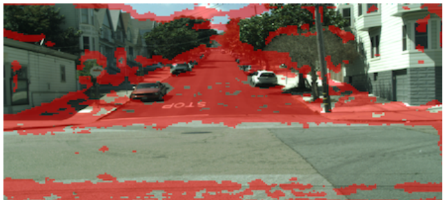
Fig. 7 Generated Stixel cuts (highlighted in red) for the FCN-based method. Stixel cut density is 31.5%, equivalent to a 3.2\times reduction in vertical resolution.
