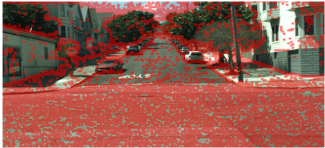
Fig. 6 Generated Stixel cuts (highlighted in red) using the left and right extrema as defined in Ignat (2016), and also cuts generated from semantic segmentation. Stixel cut density is 30%, equivalent to a 3.3\times reduction in vertical resolution.
