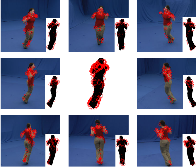
Fig. 1. Detection of STIPs in multi-frames, and extension to 4D STIPs using 3D reconstructions of the actors and pixel-to-vertex correspondences, for extraction of local 3D motion descriptors.
