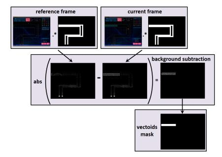
Fig. 3: Background subtraction Process
