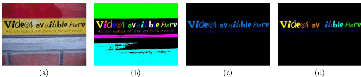
Figure 4.5: A natural scene image from the ICDAR2003 dataset (a) with its MSER decomposition (b), and the maximal meaningful clusters in feature spaces #1 and #7 of Table 4.1 (c) and (d).
