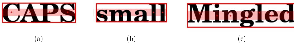
Figure 4.10: Distribution of the character centres y-coordinates in a text line: a valid text line can be characterized by its mean and Coefficient of Variation.
