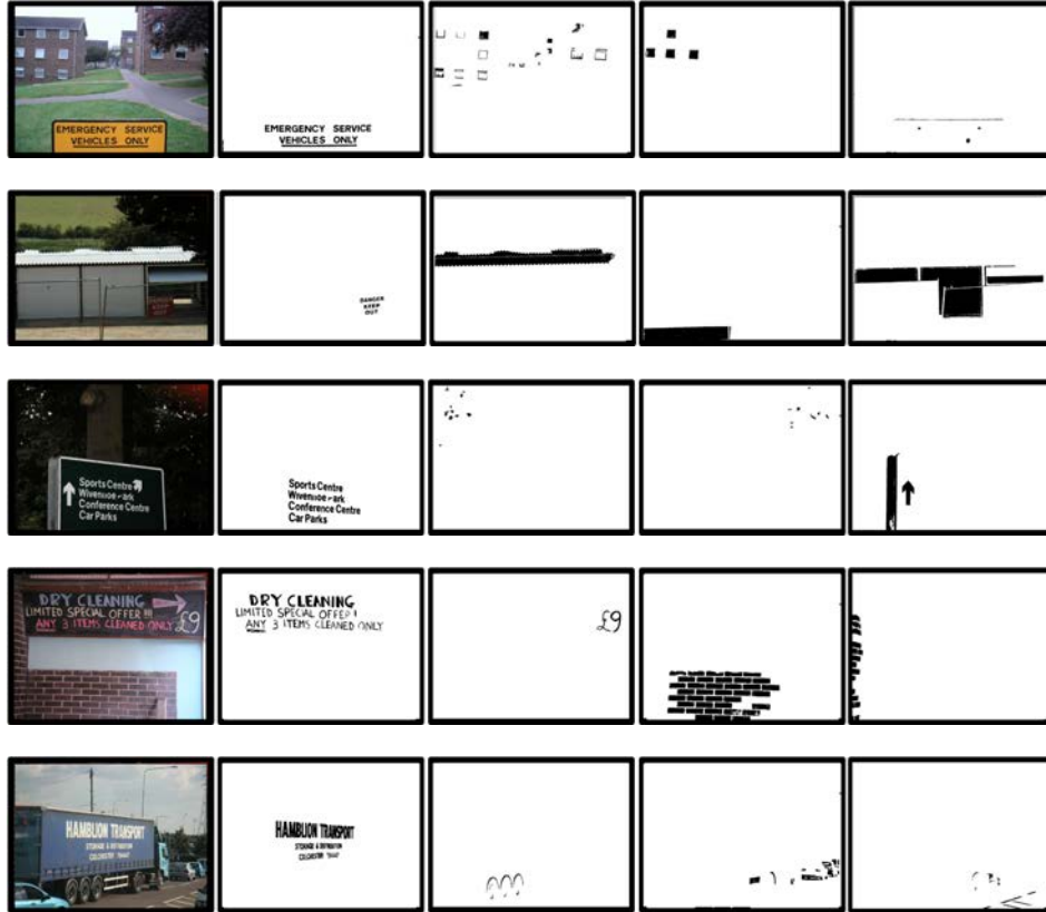
Figure 4.8: Resulting clusters of the Perceptual Organization Clustering method in natural scene images from the ICDAR2003 dataset.
