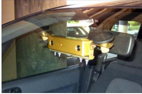
Figure 8: Stereo pair used in our acquisition system.
