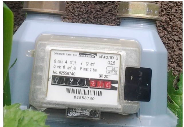
Figure 3. Utility meters may have different reading lengths depending on the model. This particular model has 5 significant digits followed by three non-significant digits (in red) that correspond to the decimal part of the reading. The ground-truth data for this image would be the string "01971". Image source: Wikimedia Commons CC-BY-SA-3.0.
