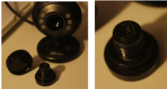
(a) IR-only filter, camera lens and camera body
