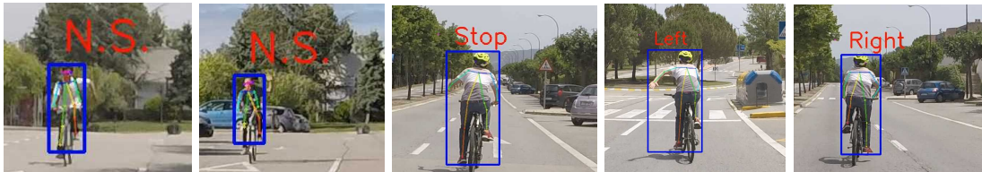
Fig. 14: Wrong predictions in CASR for cyclist indications (cropped from the original images). 'N.S.' stands for no sign .
