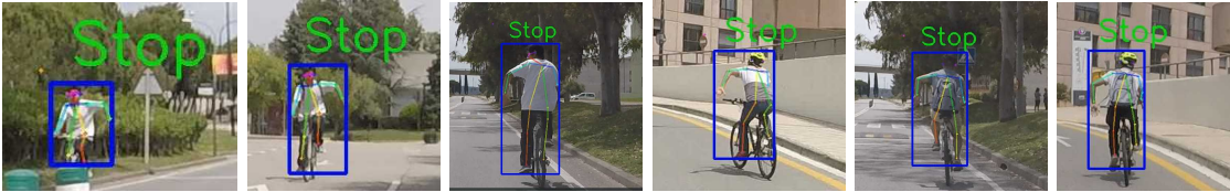
Fig. 12: Examples of correct predictions in CASR for cyclist stop indications (cropped from the original images).
