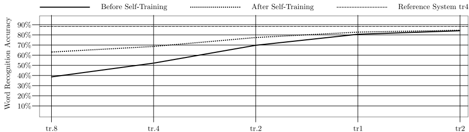
Figure 8: The initial recognition accuracy and the final recognition accuracy after 3 iterations of self-training.
