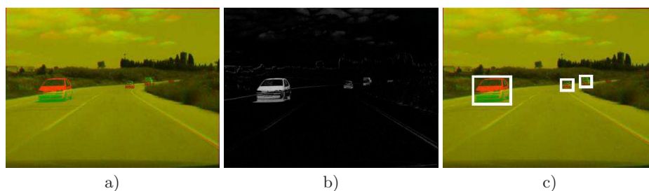
Fig. 4. Video alignment results: a) fusion, b) absolute difference, c) pre-detection of vehicles. Results in video form can be properly viewed at www.cvc.uab.es/ADAS/projects/sincro/ECCV08Workshop/ .
