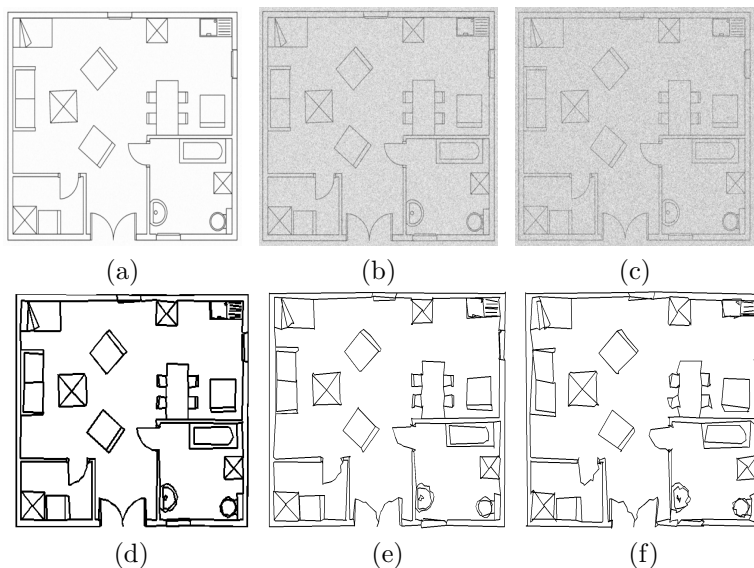
Figure 8: Examples of degraded floorplans. (a)-(c) The same floorplan in Figure 7b degraded with Gaussian noise ( m=0.1, \sigma=0.01 ), ( m=0.3, \sigma=0.05 ) and ( m=0.5, \sigma=0.09 ) respectively, (d)-(f) The same floorplan in Figure 7b degraded with vectorial noise r=5, 10 and 15 respectively.
