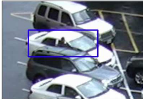
Figure 7: Activity “getting into vehicle”, where the human is occluded by other cars and the activity is hardly visible. Due to this occlusion not enough motion features are obtained and hence, overall detection performance suffers.
