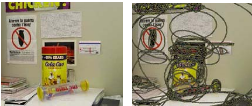
Figure 6.7: Examples of region detection. We can group the parts of the bomb drawing or the textures of the background posters.
