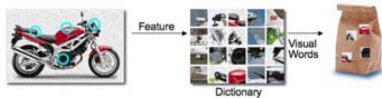
Figure 2.39: Bag of words strategy defines a dictionary of image parts and represents an object as a collection of them. (reprinted from [Woj09])
