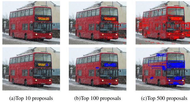
Fig. 6. The top-N hypotheses generated by the baseline Text Proposals method (top row) and after re-ranking using the mean text probability (bottom row).
