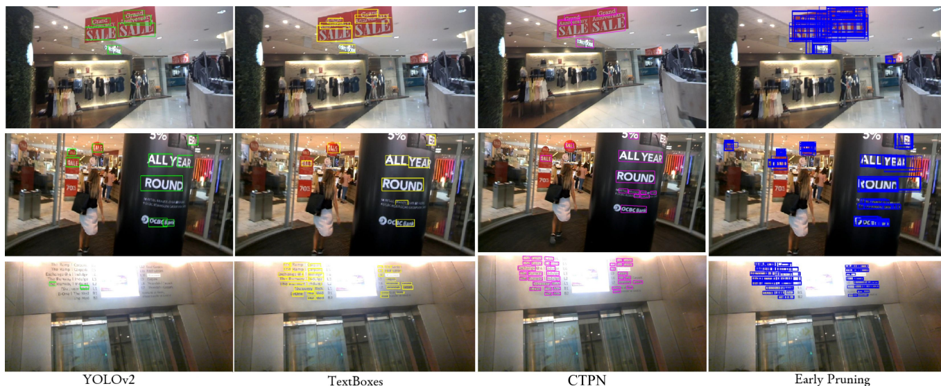
Fig. 9. All true hypotheses generated (matching ground truth regions with \text{IoU} > 0.5 ). Text Proposals with Early Pruning hypotheses are shown in blue, TextBoxes in yellow, YOLOv2 in green and CTPN in purple. Small text seems to pose problems for YOLOv2, CTPN and TextBoxes, but not for Text Proposals with Early Pruning.
