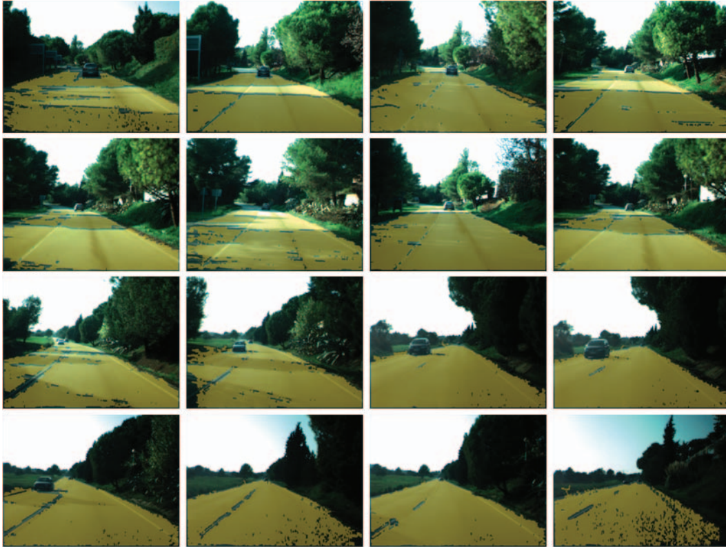
Figure 3. Results of the proposed algorithm to detect roads.
